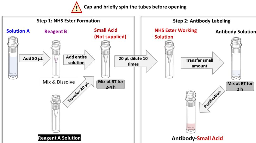
**Scheme 1.** Schematic diagram of the workflow for preparing antibody-small molecule conjugates starting with 3 mg of IgG (volume of reagents varies if the amount of IgG is < 3 mg).
