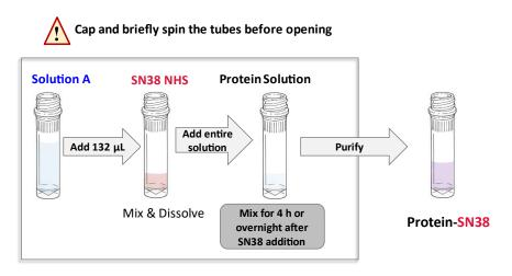
**Scheme 1**. Schematic diagram of the workflow for preparing Protein–SN38 conjugates starting with 20 nmol of Protein (volume of reagents varies if the amount of Protein is < 20 nmol and the MW is <60 KDa).
