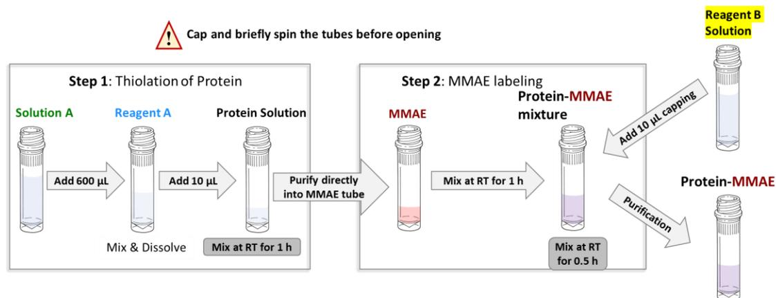
**Scheme 1.** Schematic diagram of the workflow for preparing protein-MMAE conjugates starting with 20 nmole of protein (volume of reagents varies if the amount of protein is < 20 nmole).
