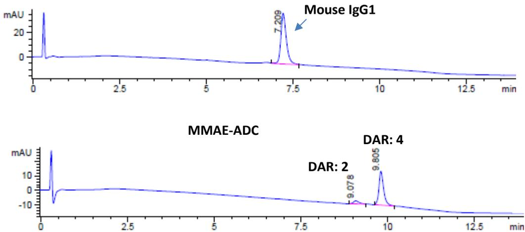
**Figure 3: SEC HPLC analysis of monoclonal mouse IgG1 and purified conjugate**
