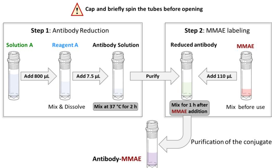
**Scheme 1.** Schematic diagram of the workflow for preparing antibody-MMAE conjugates starting with 3 mg of IgG (volume of reagents varies if the amount of IgG is < 3 mg).
