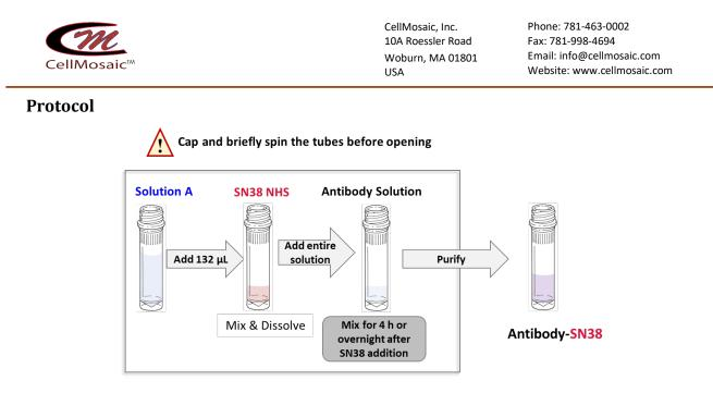
**Scheme 1**. Schematic diagram of the workflow for preparing antibody-SN38 conjugates starting with 3 mg of IgG (volume of reagents varies if the amount of IgG is < 3 mg).
